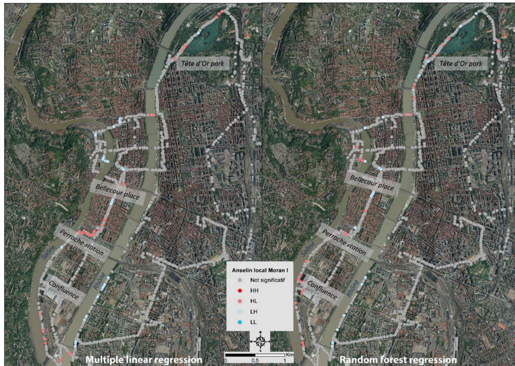
Figure 17. LISA of the differences between modelled and measured air temperatures for all study days (source: Data Grand Lyon).
