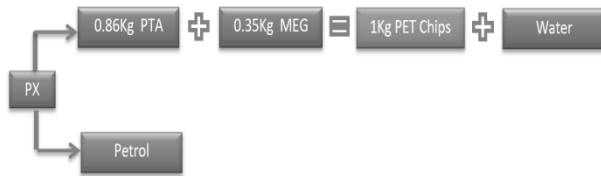
Fig. 2 -2: Relationship between PX, PTA, MEG and PET chips
